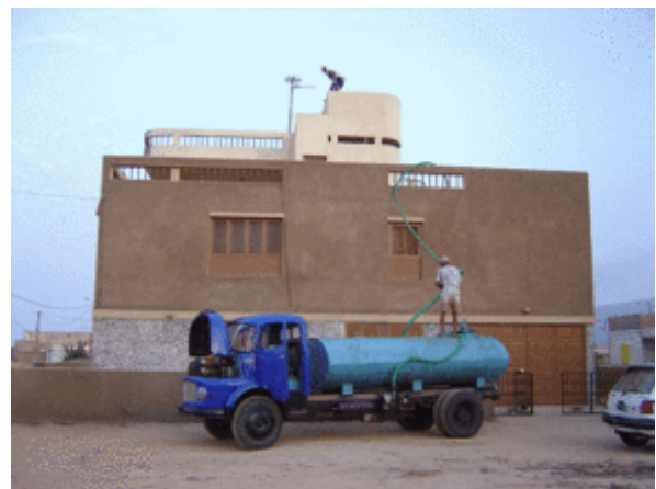
Figure 13: Autotanque for drinking water supply, in Baia das Gatas, Cape Verde
